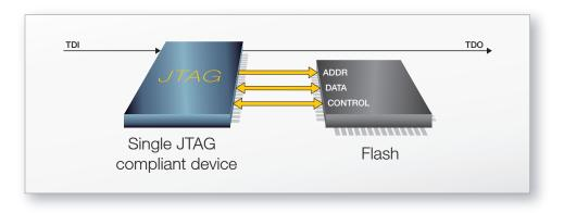
The boundary scan based in-system programming time will depend on both the length of the scan chain and the TCK frequency. For the shortest boundary scan based programming time the TCK frequency must be as high as possible and the scan chain as short as possible.
