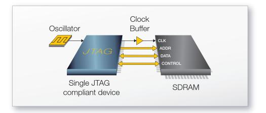
It is also important to ensure that any clock buffers do not have a minimum operating frequency. Some clock buffers have a special control input to allow low frequency signals. Such signals must be accessible from a JTAG enabled pin.
