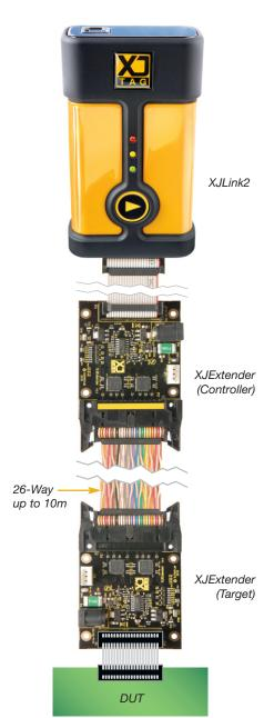
As each channel uses differential signalling, the cable generates low levels of Electromagnetic Radiation (EMR); important when testing sensitive electronic assemblies. It also exhibits very high immunity to Electromagnetic Interference (EMI), which enables the use of longer cables without loss of signal integrity.
