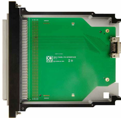
Figure 8 – Fitting the XJTAG interface board into the adapter
